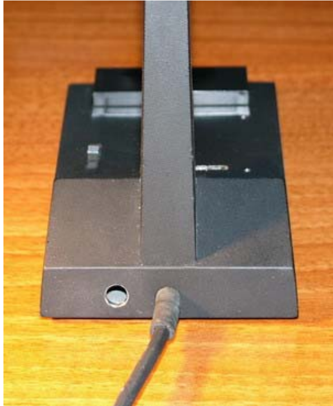
Figure 3. New cable exit hole.
